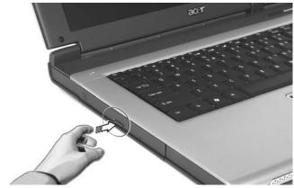
Insert a clip to the emergency eject hole to eject the optical drive tray when the computer is off.
